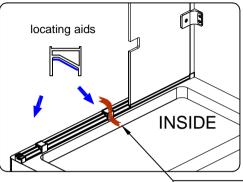
Tip! Hold both locating aids in position with masking tape.
