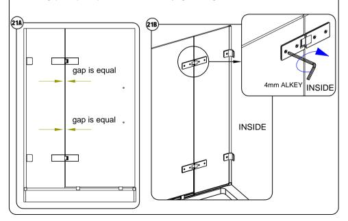
Remove spacers and check gap under moving panel is equal If gap is not equal loosen hinges slightly and adjust. Use packer to check gap is correct height and even.
