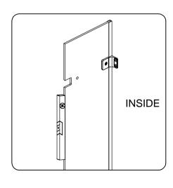
Do not fully tighten bracket to glass, leave enough slack for adjustment.
