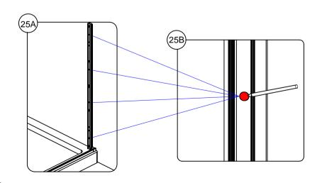
Remove profile and drill holes for wall brackets with diameter 6mm masonry bit and insert wall plugs. Make sure wall plugs are flush with tile.
