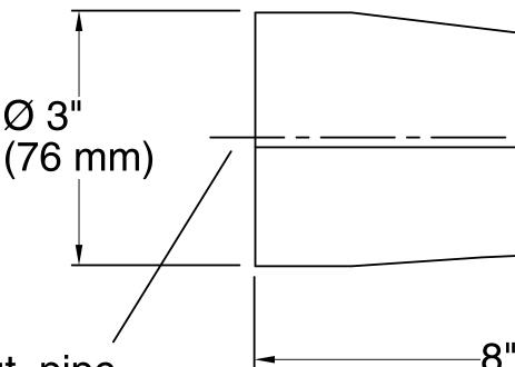
For 1/2" NPT spout, pipe must extend 7" (178 mm) beyond finished wall.
