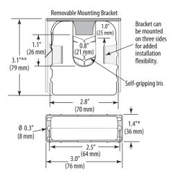
$<sup>^{\</sup>ast}\,$  Terminal block may extend up to 1/8" over the height dimensions shown.
