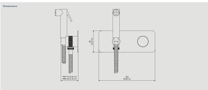
Cartridge Threaded fitting G1/2" female Ø35 ceramic cartridge Aerator Flow Rate (+/-10%) 3 BAR 1 BAR 2 BAR
