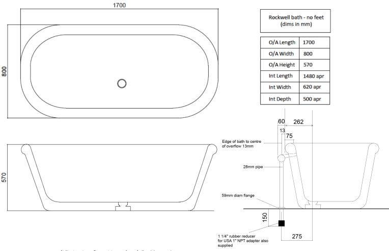
Waste:  $1 \frac{1}{2}$  BSP; Overflow: 28mm /  $1 \frac{1}{4}$  rubber reducer. We only supply fittings above the floor. We do not supply the trap; the trap needs to go beneath the floor. Dimensions are given in mm, they are a guide only and may vary from bath to bath.
