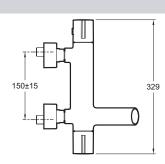
Product Specification: Thermostatic single-lever wall-mount bath/shower mixer. E8992. Collection: TOOBI. WEIGHT: 3.2 kg. MATERIAL: 54. INSTALLATION TYPE: 2 holes. TYPE: Single-lever. FLOW RATE: 19 I/min. CONNECTION: With connectors and wall escutcheons. MECHANISM: Expanding wax thermostatic cartridge. SAFETY STOP: 40°C. WARM BODY: Yes. NON-RETURN VALVE: Yes. DIVERTER: Automatic diverter built into flow handle. MECHANISM GUARANTEE: 5 years. Safety stop at 37°n.
