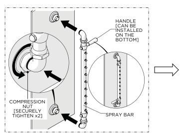
Place the BAR over the COPPER SUPPLIES then thread and securely tighten the COMPRESSION NUTS onto the BAR.
