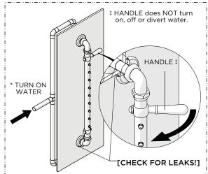
Turn on the water and a diverter/wall valve (sold separately) to flush out any debris in the supply line, operate the HANDLE to ensure it functions properly, and inspect all connections for leaks then turn the water off.
