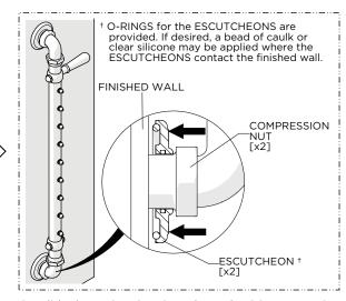
Slide the ESCUTCHEONS down the COMPRESSION NUTS until they contact the finished wall.
