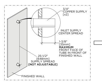
Ensure the 3/4" COPPER SUPPLIES project a maximum of 1-3/8" [35mm] from the surface of the finished wall and are at the required 25-1/2" [648mm] center spread.
