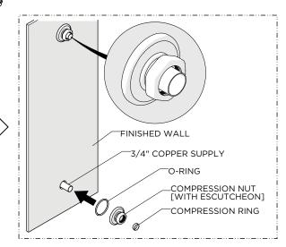
Slide the O-RING, COMPRESSION NUTS with the ESCUTCHEONS, and COMPRESSION RINGS onto the COPPER SUPPLIES.
