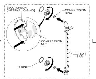
Slide the ESCUTCHEONS up the COMPRESSION NUTS then unthread and remove the NUTS from the SPRAY BAR. Do NOT discard the O-RINGS or COMPRESSION RINGS.
