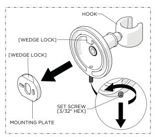
Loosen, but do NOT remove, the SET SCREW on the bottom of the HOOK using a 3/32" HEX KEY and remove the MOUNTING PLATE.
