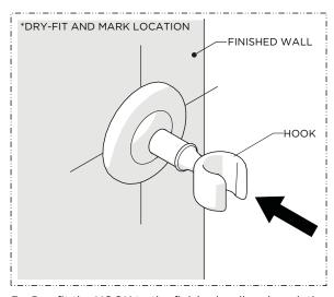
Dry-fit the HOOK to the finished wall and mark the ideal location for installation; preferably over adequate blocking or stud material.
