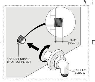
Ensure the 1/2" NPT NIPPLE (not supplied) is 5/8" [16mm] from the surface of the finished wall then thread and securely tighten the SUPPLY ELBOW onto the NIPPLE.
