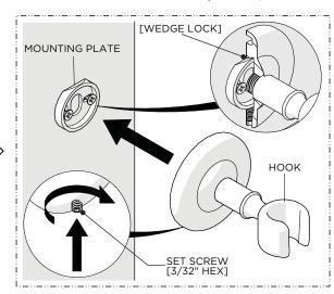
Place the HOOK over the MOUNTING PLATE then securely tighten the SET SCREW.
