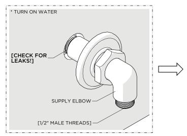
7. Turn on the water and a diverter/wall valve (sold separately) to flush out any debris in the supply line and inspect all connections for leaks then turn the water off.
