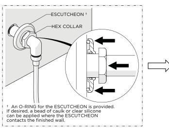
10. Slide the ESCUTCHEON and HEX COLLAR down the SUPPLY ELBOW until they contact the finished wall.
