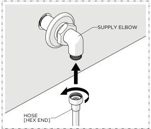
8. Thread and securely tighten the hex end of the HOSE to the ELBOW.
