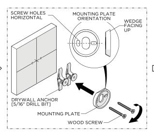
Using the previous marks as a reference, install the MOUNTING PLATE using the ANCHORS (if needed) and WOOD SCREWS provided.
