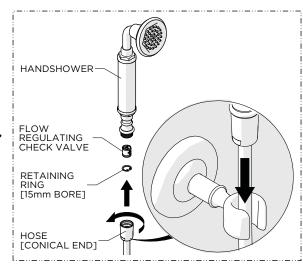
9. Thread and securely tighten the conical end of the HOSE to the HANDSHOWER then place it into the HOOK.
