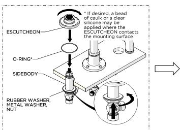
4. Thread the ESCUTCHEON back onto the SIDEBODY until it stops, and let it rest on the mounting surface. Hand tighten the NUT against the underside of the mounting surface.
