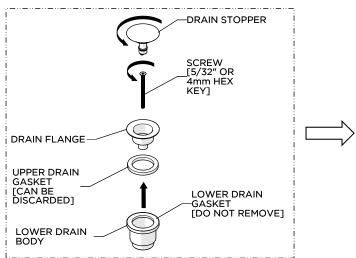
Unthread and remove the DRAIN STOPPER and LOWER DRAIN BODY from the DRAIN FLANGE The UPPER DRAIN GASKET can be discarded.
