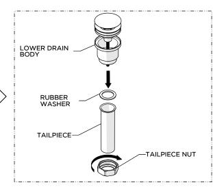
Remove the TAILPIECE from the LOWER DRAIN BODY.
