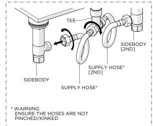
Connect the SIDEBODIES to the TEE using the SUPPLY HOSES provided. Securely tighten the HOSES and ensure they are not pinched/kinked.
