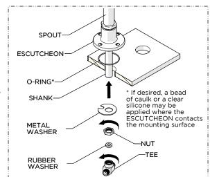
Insert the SHANK through the hole on the mounting surface and re-attach the WASHERS, NUT, and TEE. Securely tighten the NUT and TEE.
