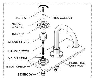
5. Place the HANDLE STEM on the VALVE STEM, then place the GLAND COVER onto the ESCUTCHEON, making sure it is fully seated. Install the HANDLE on the HANDLE STEM in the desired orientation and secure with SCREW, making sure to include the METAL WASHER AND HEX COLLAR. DO NOT tighten SET SCREW at this time.
