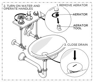
15. Removed the AERATOR, turn on the water to flush out the supply lines, and inspect all connections for leaks. Close the DRAIN to ensure it functions properly then turn off the water and re-install the AERATOR.
