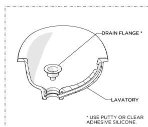
Set the DRAIN FLANGE in the lavatory [SOLD SEPARATELY] using putty or a clear adhesive silicone.
