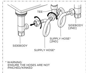
8. Connect the SIDEBODIES to the TEE using the SUPPLY HOSES provided. Securely tighten the HOSES and ensure they are not pinched/kinked.
