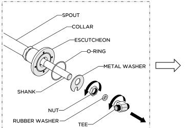
Remove the TEE, NUT and lower deck WASHERS from the SPOUT SHANK. Do NOT remove the O-RING from the ESCUTHCEON.
