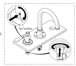
Ensure the HANDLE is in the desired orientation then securely tighten the NUT on the SIDE BODY. Align the GLAND COVER as shown then securely tighten the SET SCREW.
