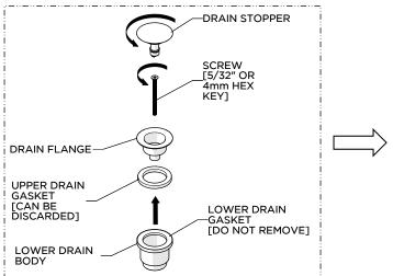
Unthread and remove the DRAIN STOPPER and LOWER DRAIN BODY from the DRAIN FLANGE The UPPER DRAIN GASKET can be discarded.
