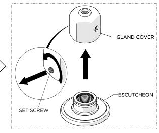
Unthread, but do not fully remove the SET SCREW, then detach the GLAND COVER from the ESCUTCHEON.
