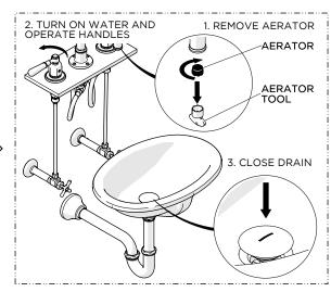
15. Removed the AERATOR, turn on the water to flush out the supply lines, and inspect all connections for leaks. Close the DRAIN to ensure it functions properly then turn off the water and re-install the AERATOR.
