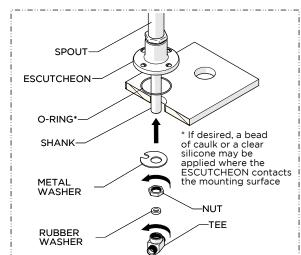
Insert the SHANK through the hole on the mounting surface then re-attach the WASHERS, NUT, and TEE and securely tighten the NUT.
