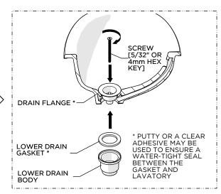
12. Re-install the LOWER DRAIN BODY making sure to use the GASKET provided. Ensure the GASKET makes a full seal on the underside of the lavatory then securely tighten the SCREW.
