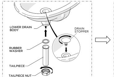
13. Re-install the DRAIN STOPPER then the TAILPIECE using the WASHER and NUT provided.
