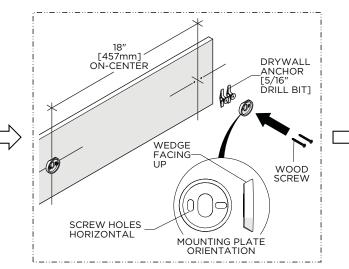
4. Using the previous marks as a reference, install the MOUNTING PLATES using the SCREWS and ANCHORS provided.
