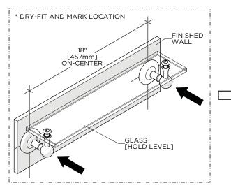
3. Dry-fit the product to the finished wall and mark the ideal location making sure to hold the product level.
