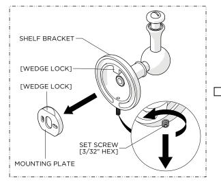
Loosen, but do <u>NOT</u> remove, the SET SCREW on the bottom of each SHELF BRACKET using a 3/32" HEX KEY and remove the MOUNTING PLATES.
