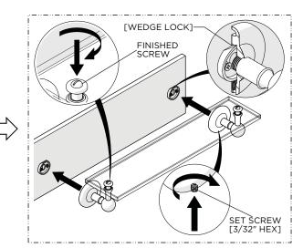
Place the BRACKETS over the MOUNTING PLATES and securely tighten the SET SCREWS FINISHED and FINISHED SCREWS.
