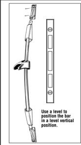
Slide the upper bracket cover onto the bar and mount bar on lower wall bracket. Using a level, position the bar in a level vertical position and mark the drill holes. Move the bar slightly out of the way and drill the holes. Insert anchors or toggle bolts and, with the wall bar attached, position the wall bracket over the holes. Insert and tighten the screws.
