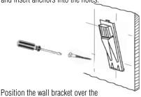
holes, insert and tighten the screws.
