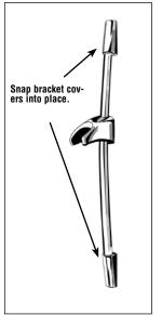
Slide each bracket cover over its respective wall bracket and snap them into
