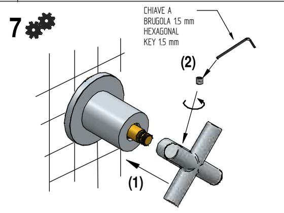
**⚠ SOSTITUZIONE VITONE / CERAMIC VALVE REPLACEMENT**
