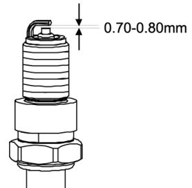
**Note:** The engine must be cold
