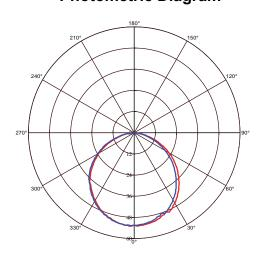
C0 Plane beam angle(50%):110.4(DEG) C90 Plane beam angle(50%):109.6(DEG)
