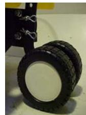
Then fit the depth skid and wheel clamp using the two cotter bolts supplied.
