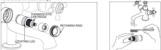
The concealed thermostatic cartridges should give trouble free service, but in the event of failure, servicing is straight forward. A) Remove the cartridge retaining ring.
