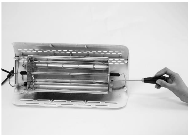
3. REMOVE THE FRONT COMPONENT OF THE DEVICE. UNSCREW THE SCREWS OF THE CLAMPS TO WHICH THE TWO BULB CORDS ARE CONNECTED.
