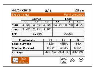
**THDi**: Total Harmonic Distortion of the current as a percentage of fundamental per phase at the Source and the Load.
