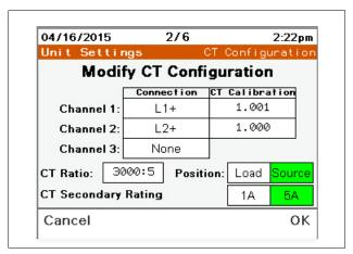
2. Once the unit is properly configured for the CTs that are installed, press OK to continue.
