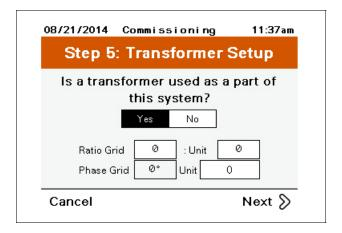
3. Change the settings on the External Transformer screen if there is a external transformer between the active harmonic filter and the voltage bus being corrected.
