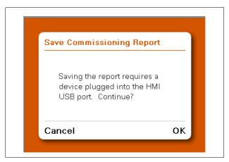
4. Press OK when USB storage device is installed.
