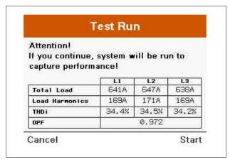
When the test run has completed, the unit or system performance results are displayed. You should see a significant reduction in THDi between Unit On versus Unit Off.
