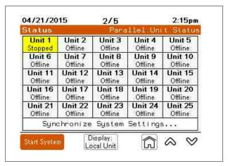
The Parallel Unit Status provide general operating condition of each unit in the parallel system.
