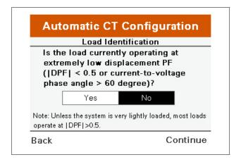
2. Touch Yes or No as applicable for the connected loads and then touch Continue. The unit asks if the connected load at the time of the CT detection was capacitive (having a leading power factor) or inductive (having a lagging power factor).
