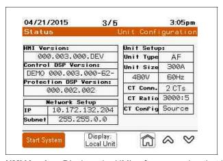
HMI Version: Displays the HMI software version that is loaded on the HMI.
