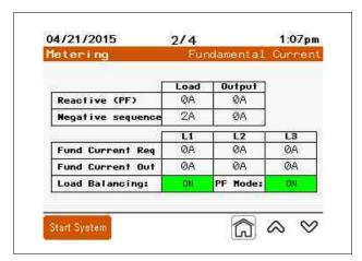
**Reactive (PF)**: Displays per phase average reactive current of the load and output in amperes RMS.
