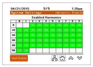
On this screen, you can select which individual harmonic orders are compensated. When ON, the harmonic order compensation is enabled. Touching any harmonic order toggles it off or on.
