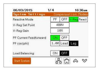
**PF Current Feedforward**: When OFF, CTs are not required for this application. The unit maintains the V - Reg Set Point based on the unit's terminal voltage.
