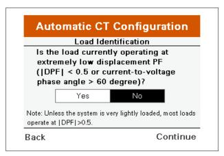
The unit asks if the displacement power factor of the load operating at the time of the test was extremely low, less than 0.5.
