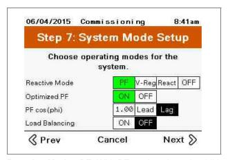
**Reactive Mode - PF**: With PF mode selected, additional parameters available for the PF mode are displayed.
