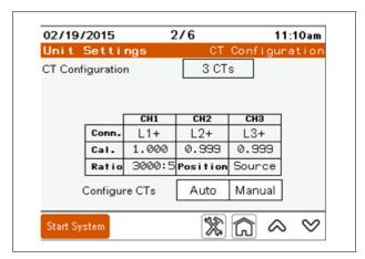
The CT Configuration screen provides information on how the unit is currently configured for the connected CTs. If needed, you can configure additional CTs manually or automatically.
