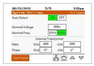
The **External Transformer** section must be changed if there is an external transformer between the active harmonic filter and the voltage bus being corrected. This parameter is not used for the integrated transformer units. These units are identified by a rating of 600 or 690 volts on the nameplate.
