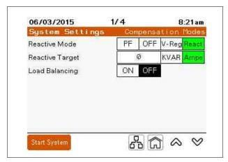
**Reactive Mode - React**: Reactive mode provides leading or lagging kVAR based on the Reactive Target. React Mode does not require the installation of CTs.
