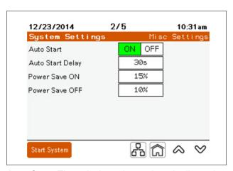
**Auto Start**: The unit shuts down when the line voltage drops below 85% of nominal. With Auto Start ON, the unit automatically returns to RUN condition when the line voltage is within 85% of nominal. The unit must be in RUN condition during the event to return to RUN condition.
