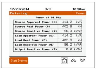
This screen displays three-phase values of the source, load, and output of the active harmonic filter.
