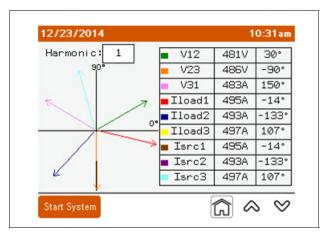
V12: Line-to-line voltage of L1 to L2.
