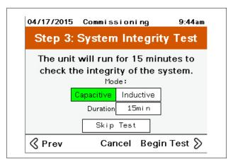
The unit can either operate in Capacitive or Inductive modes for this test. The loads operating on the system determine which mode is best for the application.
