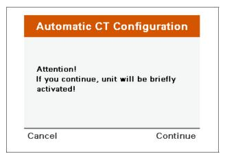
The unit runs for a short period of time to detect how the CTs are installed.
