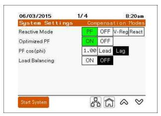
**Reactive Mode - PF**: Activates/Deactivates the Power Factor correction mode. With PF mode selected, additional parameters available for the PF mode are displayed.
