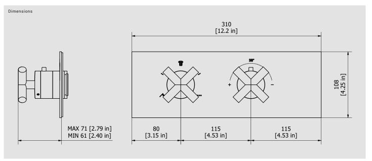
Cartridge Threaded fitting -Flow Rate (+/-10%) Aerator 1 BAR 2 BAR 3 BAR l\m l\m l\m Production Material Main body is a machined from a solid pieces BRASS According to CuZn39Pb3 (CW614N) Max Lead content: 2.5%
