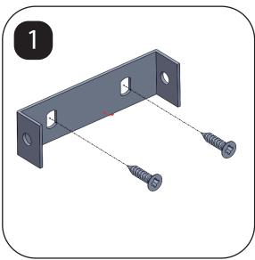
Secure the bracket to wall using screws
