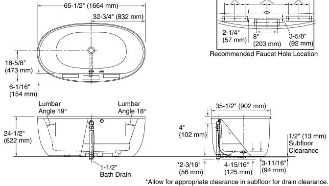
\*Allow for appropriate clearance in subfloor for drain clearance Note: Horizontal PVC pipe and tee shown, not included.
