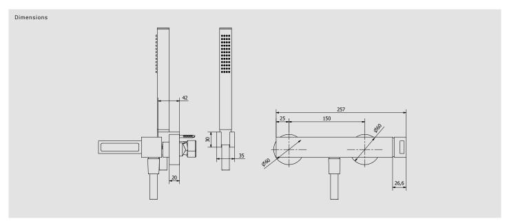
Cartridge Hoses Ceramic cartridge Ø35 Chromalux hose L150 Aerator Flow Rate (+/-10%) 1 BAR 2 BAR 3 BAR 12 I\m 17 I\m 22 I\m
