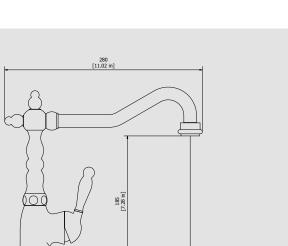
Cartridge Threaded fitting Ceramic cartridge Ø35 Inox hose M10x1 G3/8" F L400 Aerator Flow Rate (+/-10%) 1 BAR 2 BAR 3 BAR M24x1
