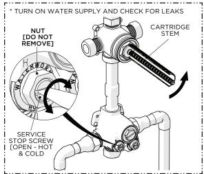
Turn on the water supplies then open the hot and cold SERVICE STOPS and operate the CARTRIDGE STEM to flush out the lines and check for leaks.
