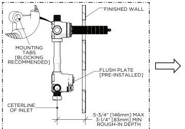
The rough-in depth is measured from the centerline of the inlets to the surface of the finished wall and must be between 5-3/4" [146mm] MAXIMUM and 3-1/4" [83mm] MINIMUM.
