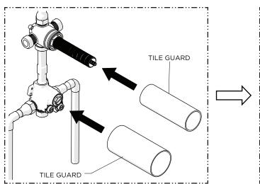
Firmly push both TILE GUARDS onto the VALVE and do NOT remove until construction is completed.
