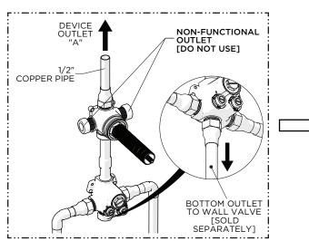
4. Run 1/2" copper lines from the VOLUME CONTROL VALVE outlet, and bottom outlet if used, to the desired end fittings (sold separately) making sure to secure all piping and fittings.
