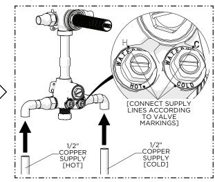
Run 1/2" copper supply lines to the proper height and depth of the VALVE INLETS making sure they are piped according to the VALVE markings and all piping and fittings are properly secured.
