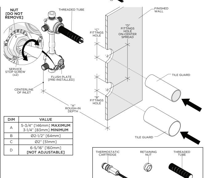
IMPORTANT: The THERMOSTATIC CARTRIDGE, RETAINING NUT, and THREADED TUBE are packaged separately and provided with the VALVE. **SET ASIDE**
