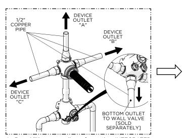
Run 1/2" copper lines from the INTEGRATED DIVERTER VALVE outlets, and bottom outlet if used, to the desired end fittings (sold separately) making sure to secure all piping and fittings.
