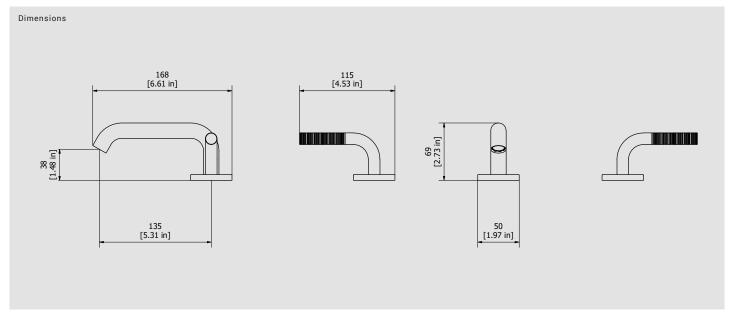
Cartridge Threaded fitting G1/2" ceramic headwork G1/2" male Aerator Flow Rate (+/-10%) 1 BAR 2 BAR 3 BAR M16.5x1 5.5 l\m 6 I\m 6 I\m
