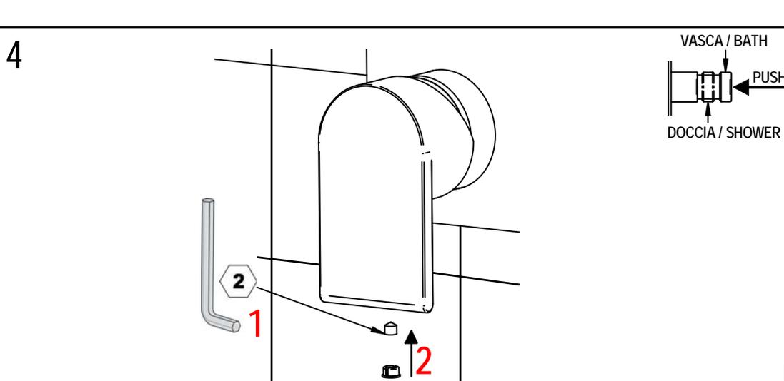
**!** **SOSTITUZIONE CARTUCCIA / CARTRIDGE REPLACEMENT**
