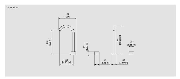
Cartridge Threaded fitting G3/8" ceramic headwork G1/2" female 400mms Aerator Flow Rate (+/-10%) 1 BAR 2 BAR 3 BAR M16.5x1 3 I\m 3.8 I\m 3.8 l\m
