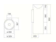
450100000 White White easy-clean (XXXX XXX 400) White antibacterial (XXXX XXX 401) without tap hole, without overflow special- or matt colour ø 325 x 900mm Glazed steel 12,4 kg for wall connection Mirror SP.300, Mirror SP.300.1, Mirror SP.325, Mirror SP.325.3, Design mirror SP.FR375.S1 Optimum point of impact approx. 116 – 146mm from rear edge of basin.
