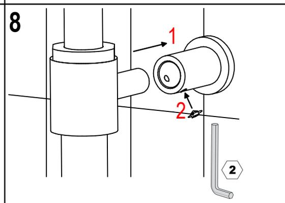
**! SOSTITUZIONE CARTUCCIA / CARTRIDGE REPLACEMENT**
