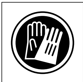
Gloves should be worn when necessary, e. g., when assembling cutting equipment.
