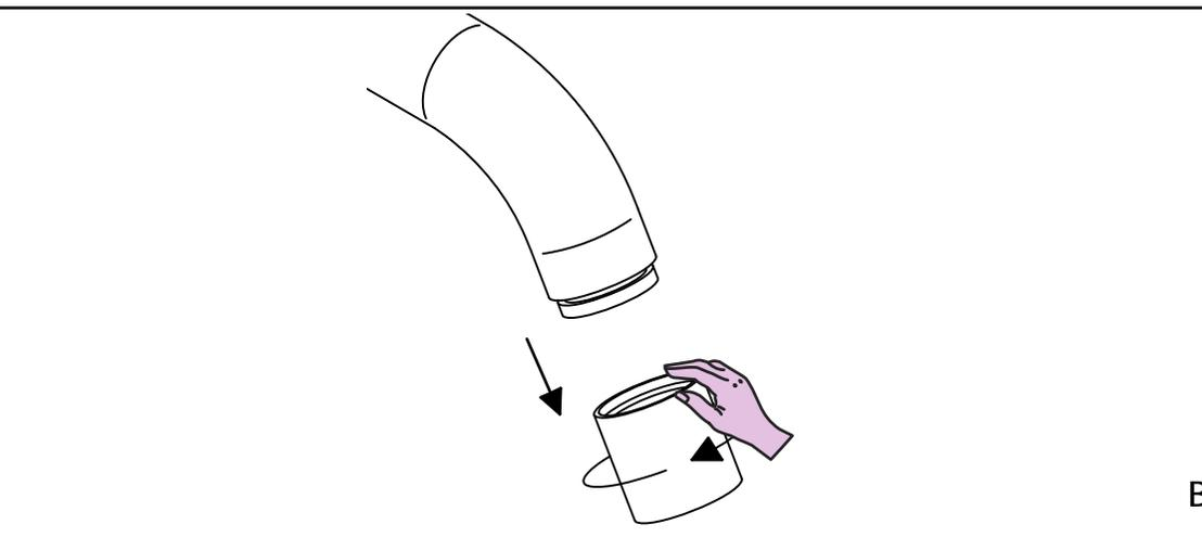
**SOSTITUZIONE SNODINO BIDET/ JOINT BIDET REPLACEMENT**
