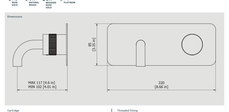
G1/2" female Ø35 ceramic cartridge Aerator Flow Rate (+/-10%)
