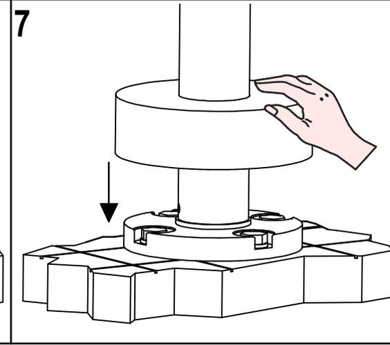
**! SOSTITUZIONE AERATORE / AERATOR REPLACEMENT**
