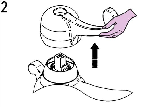
**! SOSTITUZIONE AERATORE / AERATOR REPLACEMENT**
