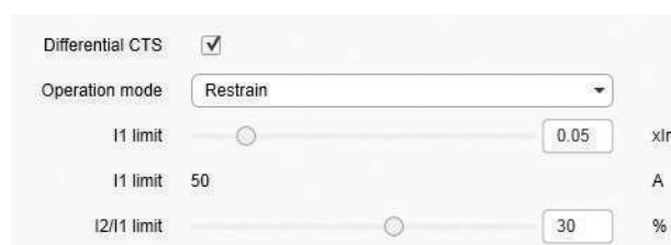
Figure 149 - Current transformer supervision settings
