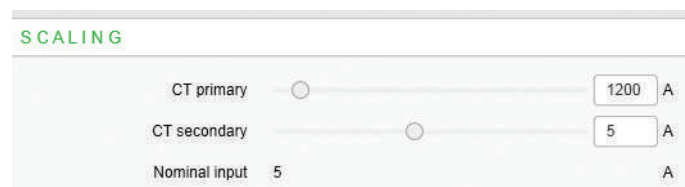
Figure 134 - Example of setting the current transformer scaling values
