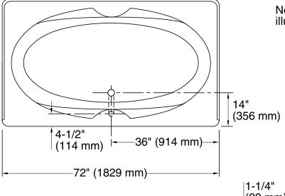
No change in measurements if connected with drain illustrated. (K-11677)
