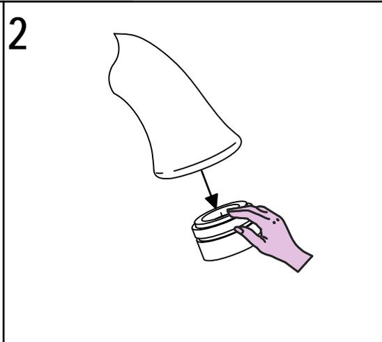
**SOSTITUZIONE SNODINO BIDET/ JOINT BIDET REPLACEMENT**
