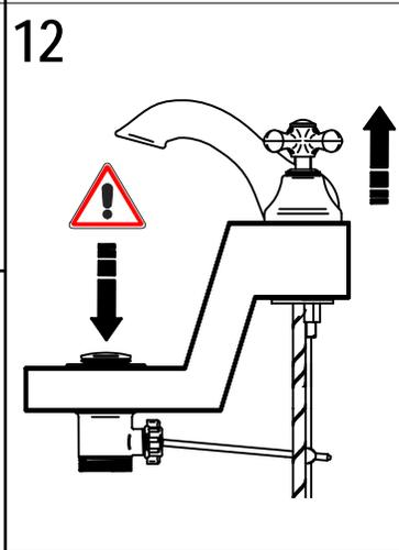
**SOSTITUZIONE AERATORE / AERATOR REPLACEMENT**
