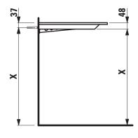
X = The exact hight must be set during installation.
