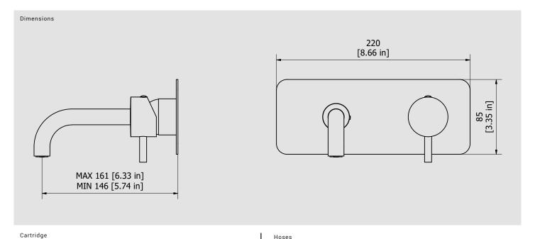
Hoses Ø35 ceramic cartridge Aerator Flow Rate (+/-10%) 2 BAR 3 BAR 1 BAR M16.5x1 10.5 l\m 7.6 l\m 13 I\m
