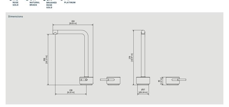
Cartridge Treaded fitting G1/2" ceramic headworks Treaded fitting G1/2" male Aerator Flow Rate (+/-10%) M16.5x1 1 BAR 2 BAR 3 BAR 4.2 I\min 5 I\min 5 I\min
