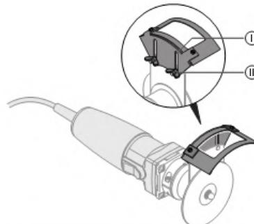
**1** Unscrew wing nuts until the protection device is loose
