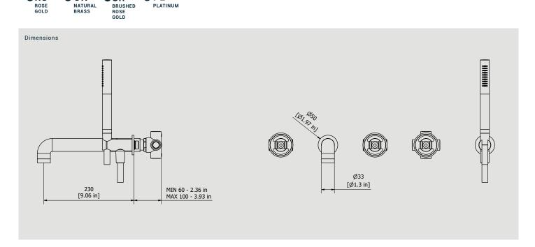
Threaded fitting Cartridge G1/2" female G1/2" ceramic cartridge
