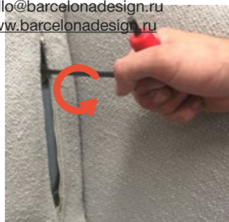
Loosen two hidden nuts in back as shown. Soltar los pasadores ocultos.
