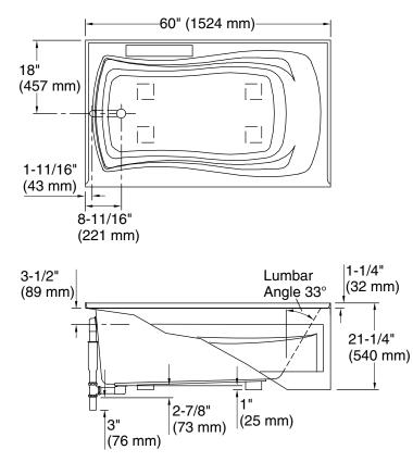
No changes in measurements if connected with drain illustrated. (K-7161-AF)
