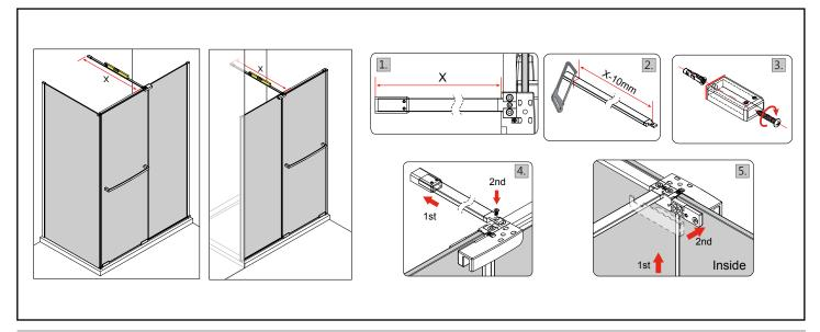
Fitting a 90 ° support bar in a recess configuration.
