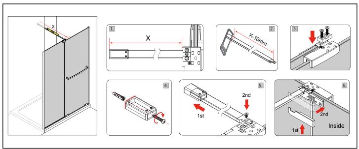
Fitting a 90° support bar and bottom track cap in a sliding shower wall configuration.
