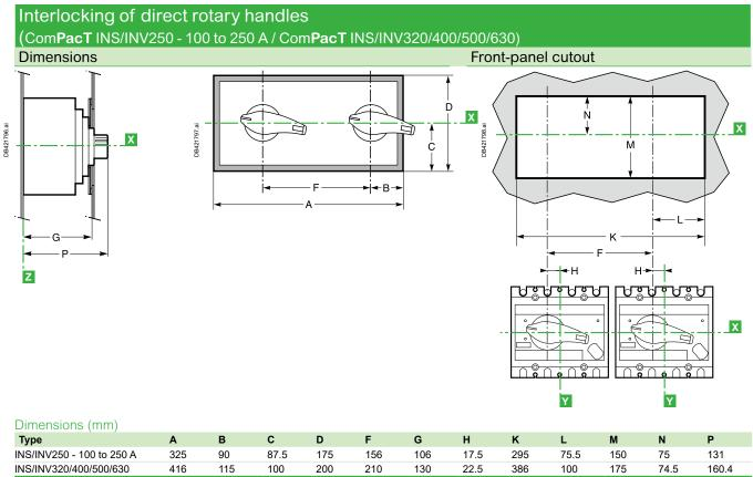
Note: X and Y are the symmetry planes for a 3-pole device.
