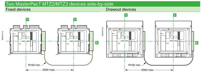
Three MasterPacT MTZ2/MTZ3 devices (switch-disconnectors or circuit breakers) side-by-side
