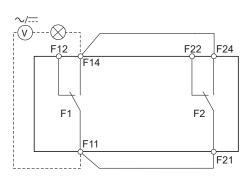
NOTE: terminal capacity for auxiliary contact is AC250 V 2 A.
