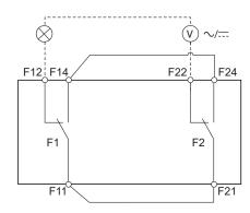
Transfer switching equipment is not at OFF position: F11-F14 and F21-F24 are closed
