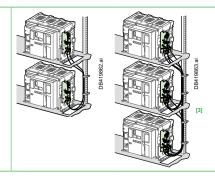
Mechanical interlocking by cables
